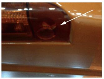
Some customers may comment on the CHMSL developing cracks in the area around the fasteners.
