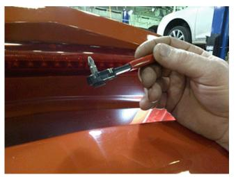
2. Remove the screws from the CHMSL. Screws were installed with Loc-Tite. Some amount of force may be necessary to loosen the screws.
