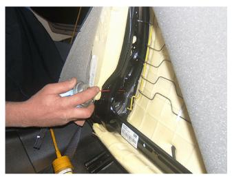
**Note:** One side latch has open access while the opposite side may have more limited access due to its location behind the seat recliner motor. Openings in the seat back frame should allow application of the spray to both the front and back side of the latches.
