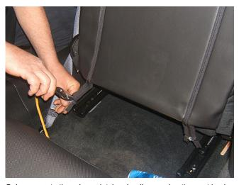
2. Gain access to the release latches by disengaging the seat back cover rear J-channel from the seat frame, then unzipping the cover on each side.
