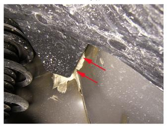
This noise may be caused by the left front plastic fender liner (splash shield) making contact with the body structure.
