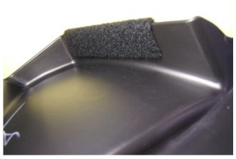
6. Fold the material length wise and install to the fender liner as shown.
