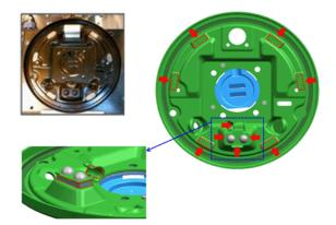
The right rear brake drum and rear brake shoes need to be replaced including applying a high temperature grease, GMP/N 12345996 (in Canada, 10953501), or equivalent, on all the locations of the backing plate as shown in the illustration above.
