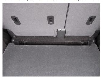
Starting with 2014 vehicle production, the floor filler trim panel was removed to increase rear stowage area. The seat/floor interface will now look like the example shown in the graphic above.
