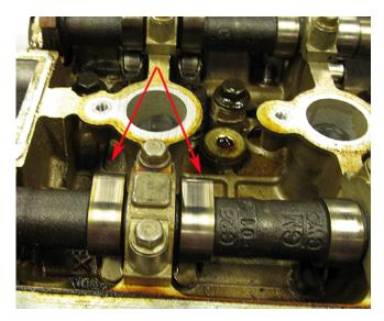
Camshafts and roller follower will have wear markings. This is normal and do not need to be replaced (refer to picture above).
