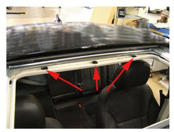
1. Remove the three hook and loop fasteners from the headliner assembly at the rear of the sunroof opening. Slide the fasteners out of the attachment slots in the headliner assembly.
