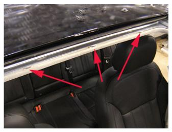
6. Install the three new service magnets in the attachment slots. Position the magnets in a fore/aft location to ensure the magnets sit flat on the sunroof housing flange.
