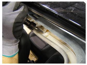
5. Use a small file or rotary bit on a die grinder to lengthen the attachment slots as shown. Use care to prevent over cutting the material.
