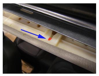
4. Using a paint pen or permanent marker, mark a 5 mm (3/16 in) area at the front edge of the three clip attachment slots as shown.
