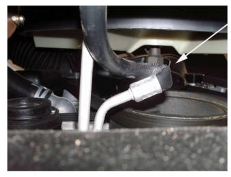
This condition may be caused by twisted or kinked transmission oil cooler lines. Inspect the transmission oil cooler lines near the radiator for any twists or kinks. Correct as required.
