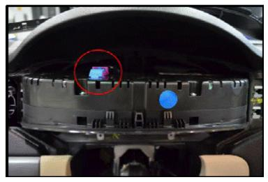
• Carefully pull the instrument cluster rearward slightly, and then tilt the assembly downward to access the wiring harness connection <circle>.
