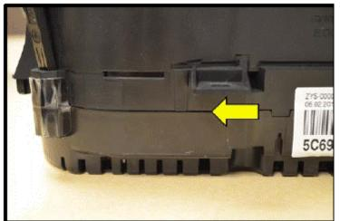
Inspect instrument cluster thoroughly to ensure both halves are fully seated and fastened together <arrow>.
