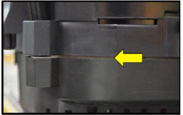
• With the instrument cluster removed from the vehicle inspect the seam between the two instrument cluster halves <arrow>.
