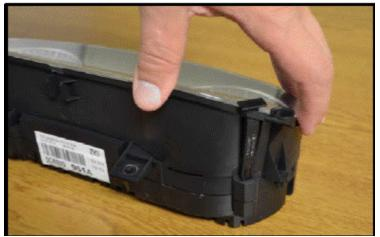
If the cluster halves are not fully seated together gently press downward on the cluster. Be sure to press on the outside edges of the lens as shown to prevent damage.
