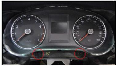
• Remove the instrument cluster mounting bolts <circles>.
