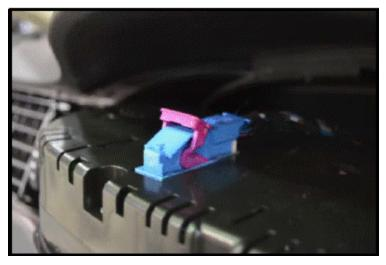
• Release the locking tab on the connector and unplug the harness from the back of the instrument cluster <as shown>.
