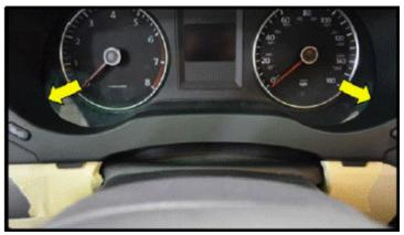
With the locking tabs in front of the knee bolster trim pull directly on the bezel by hand at the 9 o'clock, then the 3 o'clock positions of the cluster <arrows>.
