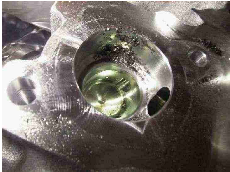
Figure 3. Metallic debris in N290 housing.
