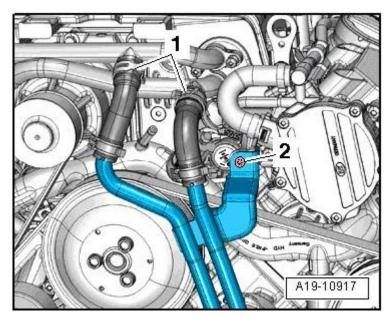
Figure 9. Bolt to be removed (2)
