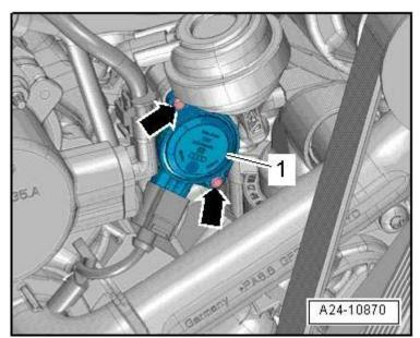
Figure 3. Intake manifold sensor (1) and bolts (arrows)
