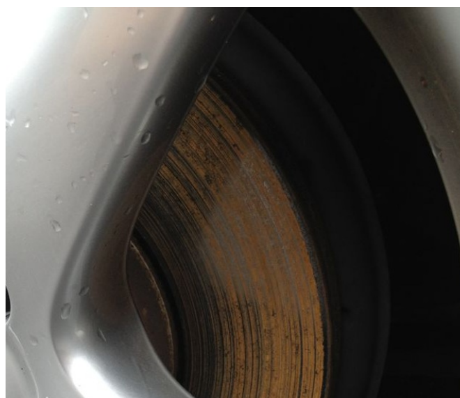
Figure 1. Disc covered with rust.
