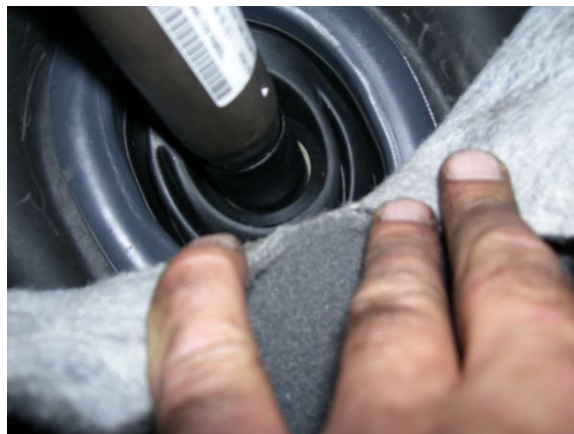
Figure 1. Sealing sleeve on the bulkhead.
