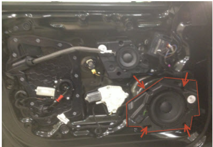
Figure 2. Front inner door panel removed, with bass speaker outlined in red.
