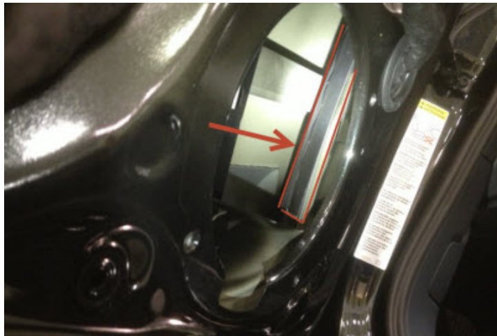
Figure 3. Access to window guide with door speaker removed.
