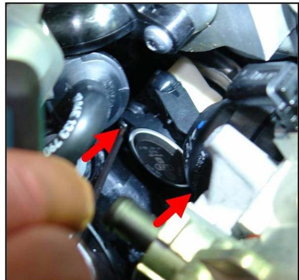
11. Pry the vacuum actuator <2> off the ball head <3>, then disconnect the vacuum hose <1>.
