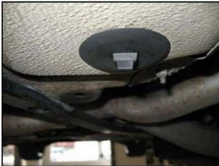
Figure 3. Installation of drain valve.
