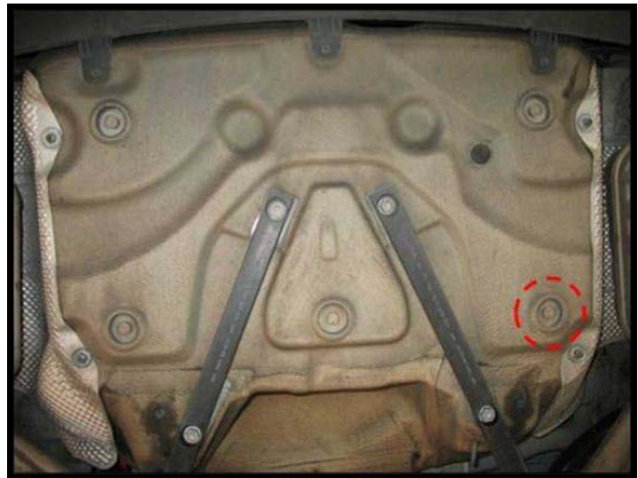
Figure 1. Red circle indicates the sealing cap that is stuck to the right side of the battery recess.
