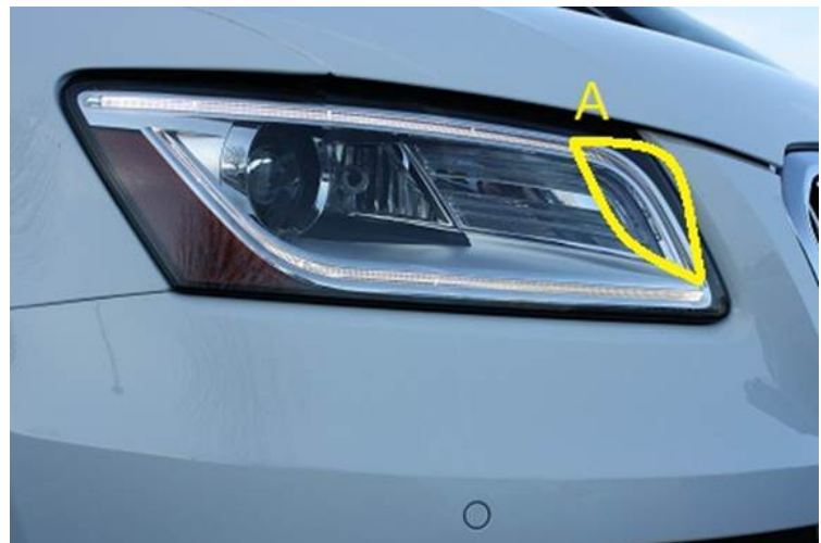
Figure 4. Upper light pipe perceived defect (A).
