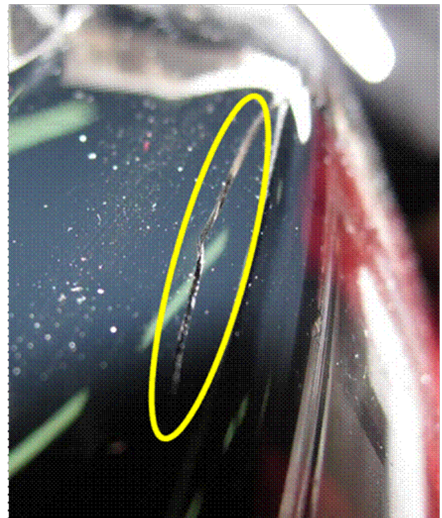
Figure 4. Upper headlight housing cracking.
