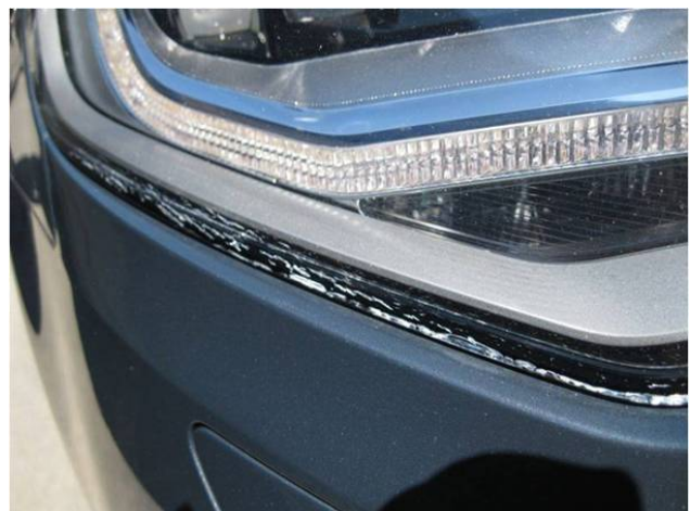
Figure 2. Lower headlight lens cracking.
