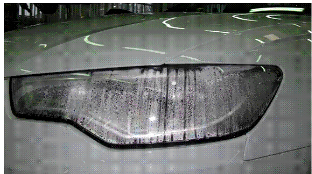
Figure 1. Headlight with heavy condensation
