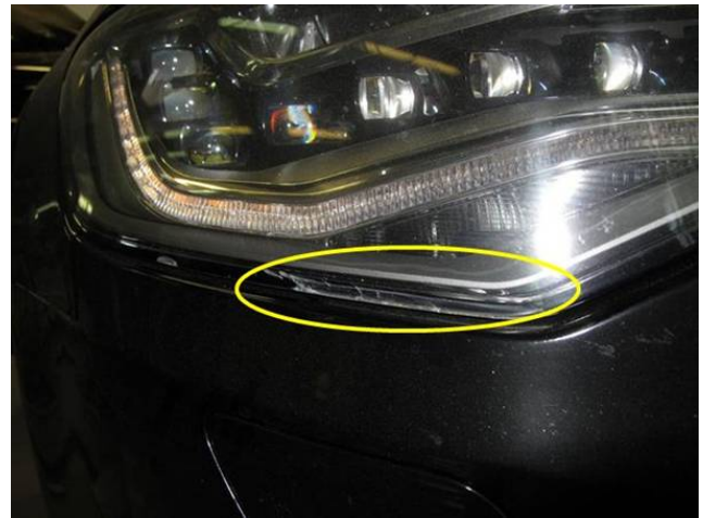
Figure 3. Lower headlight lens cracking.
