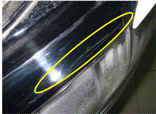
Figure 5. Upper headlight housing cracking.
