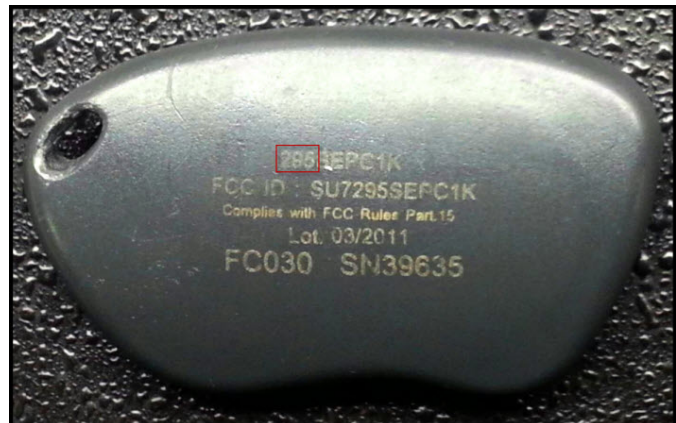
Figure 2. Stingray Transmitter (back view) with model number 295SEPC1K, where “295” denotes the operational frequency.
