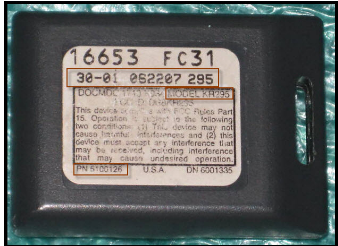
Figure 1. Sentex Transmitter (back view) with model number KR295, where “295” denotes the operational frequency.
