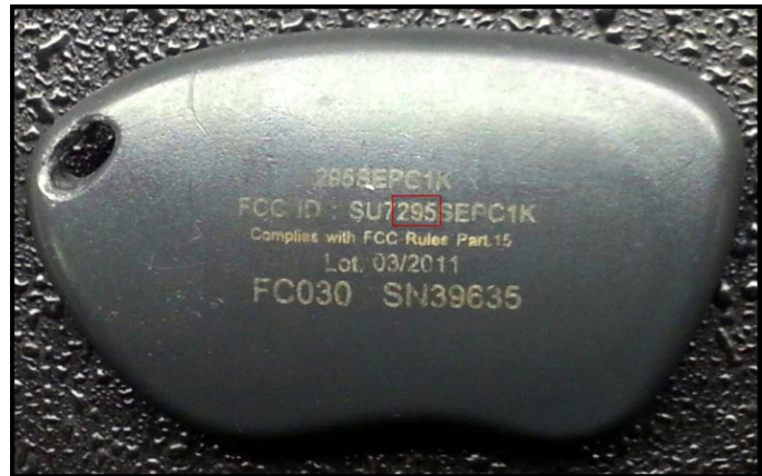
Figure 3. FCC ID is listed as “SU7295SEPC1K”, where “295” indicates the transmitting frequency.
