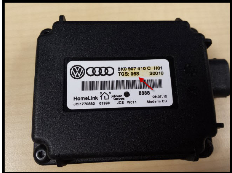
Figure 5. Locating the TGS level on the part label. This example shows part number 8K0907410C, with TGS level 06S.
