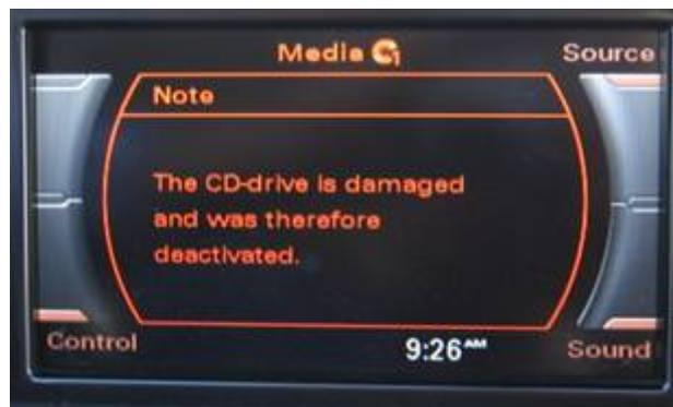
**Figure 2.** The “damaged CD drive” error message.
