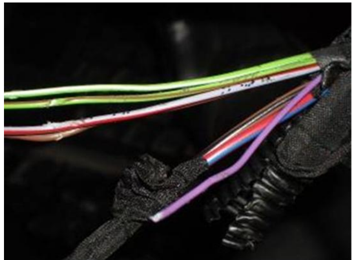
Figure 2. Wire harness under driver's side headlight.
