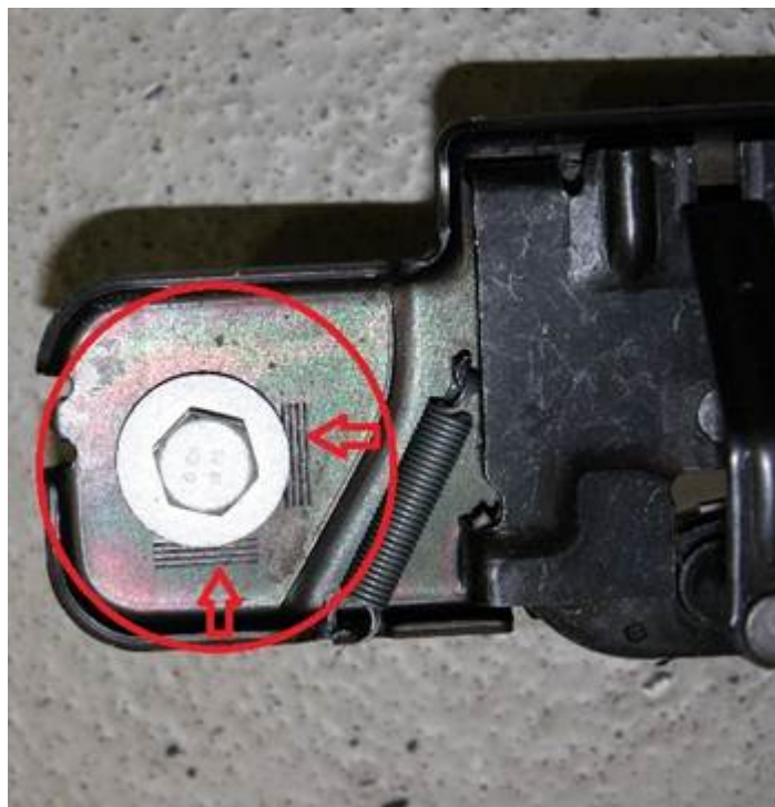
Figure 5. Power lid's motorized striker plate adjustability and serrated indicators.
