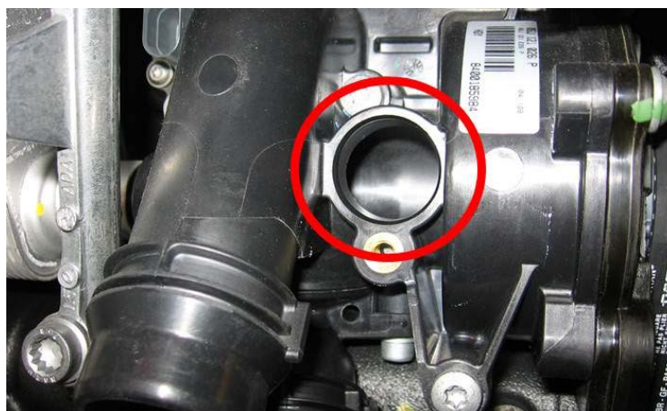
Figure 1. Connection of water pump and hose leading to heater core
