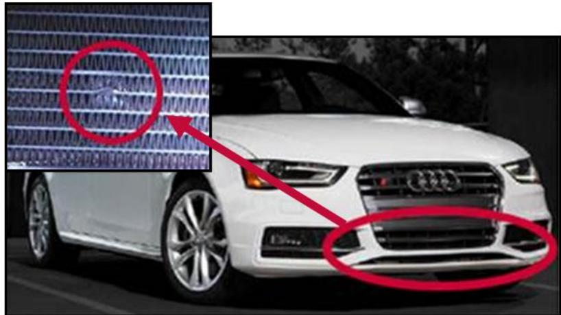
*Figure 1. Damage from front-end stone impact.*
