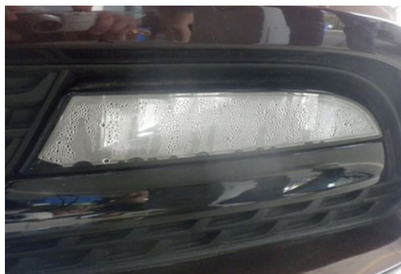
Figure 1. Fog lamp with a significant amount of standing water at the base of the lens.
