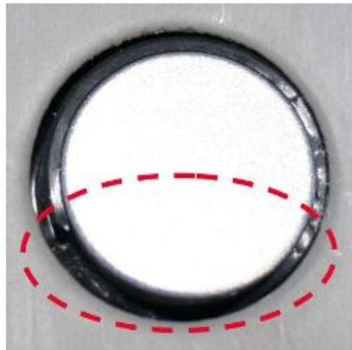
**Figure 5.** An incorrectly seated decoupling ring (folded).
