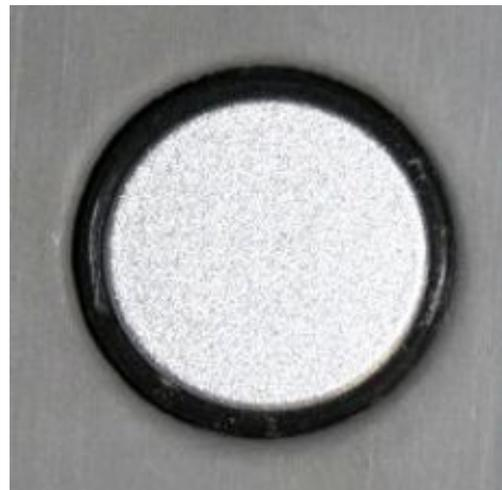
**Figure 3.** A correctly seated decoupling ring.
