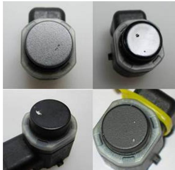
**Figure 1.** Stone chips causing sensor failure.
