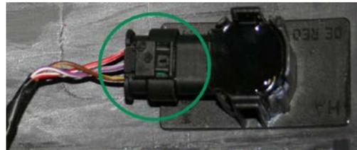
**Figure 12.** A correctly installed parking aid sensor connector.
