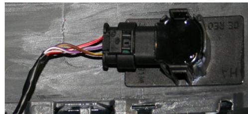
**Figure 10.** A correctly installed cable with sufficient length.
