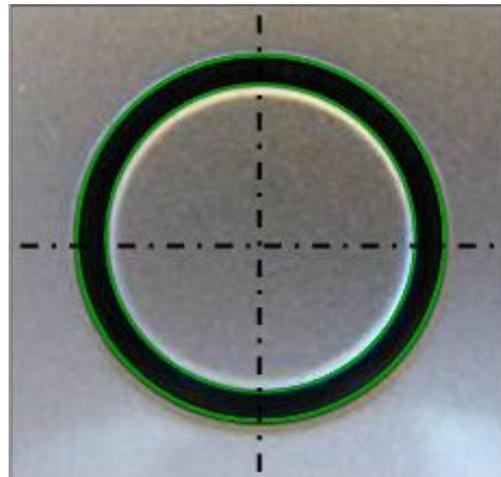
**Figure 6.** A correctly centered parking aid sensor.
