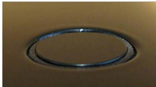
**Figure 8.** A correctly installed parking aid sensor.
