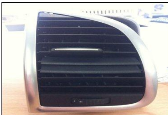
Figure 1. Damaged fins on an outer instrument panel vent.
