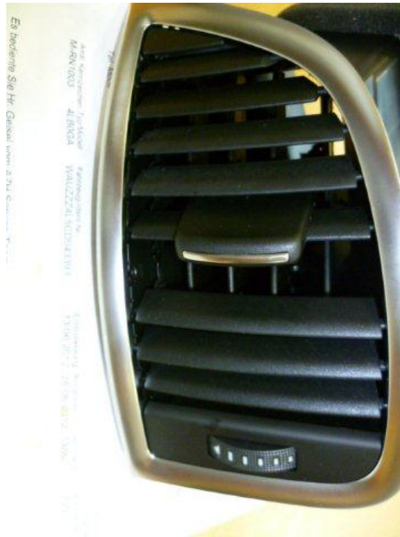
Figure 2. Missing fins on an outer instrument panel vent.
