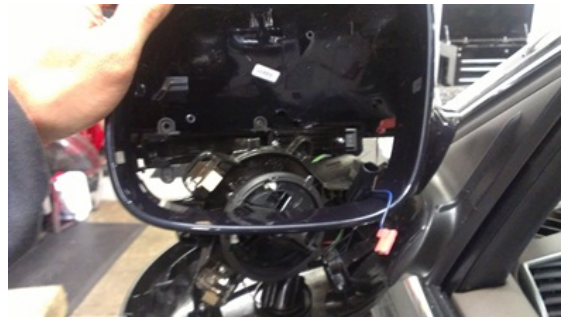
Figure 2. Removal of the mirror housing from the mirror base.
