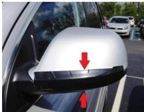
Figure 1. Application of tape over turn signal lamp.
