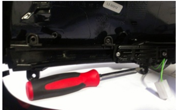
Figure 2. Removal of the mirror housing from the mirror base.
