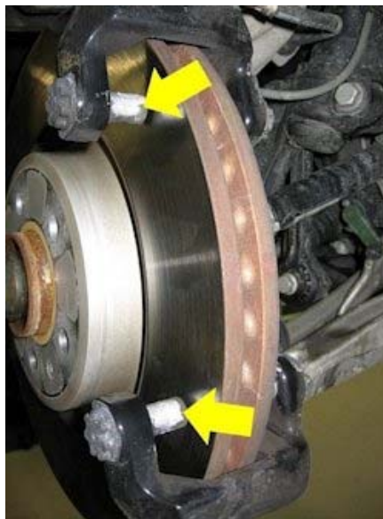
Figure 5. Caliper carrier guide pins with anti-seize ( G 052560A2 ) lubricant applied where the pads make contact.
