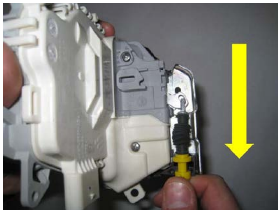
Figure 5. Pulling down the Bowden cable.
