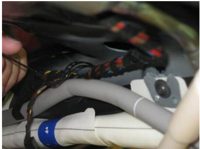
Figure 4. Open existing ties along A-pillar.
