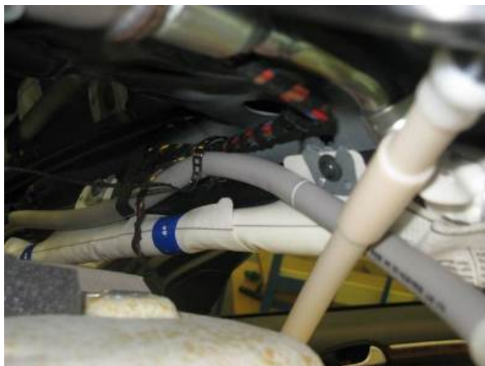
Figure 3. Open existing ties along A-pillar.
