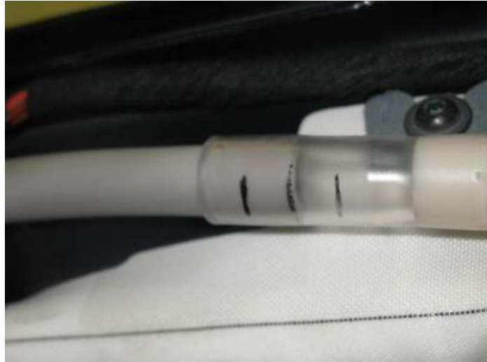
Figure 13. Lower section of hose inserted into the union.
