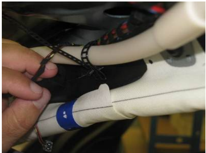
Figure 5. Routing the repair section through the cable ties.
