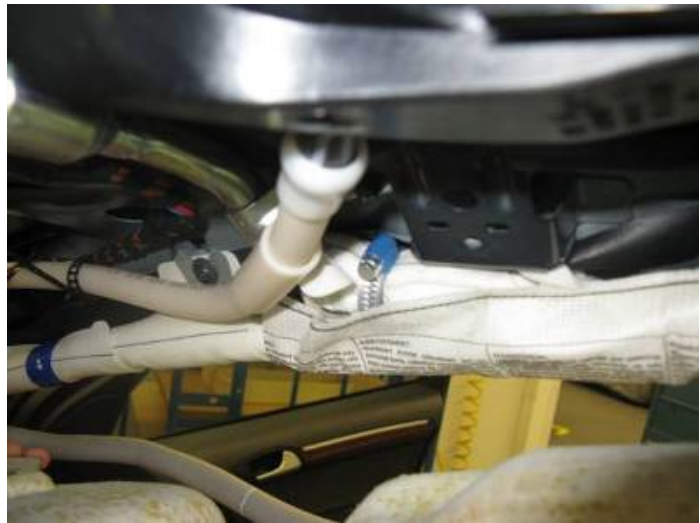
Figure 6. Routing repair section and attaching.
