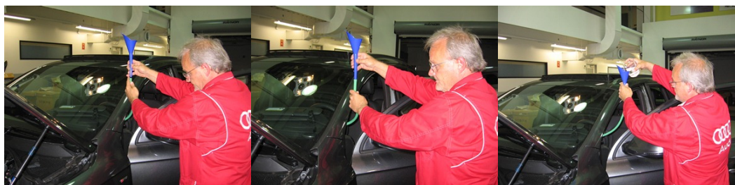
Figure 11. Fitting of the funnel and water testing the lower section of the hose.
