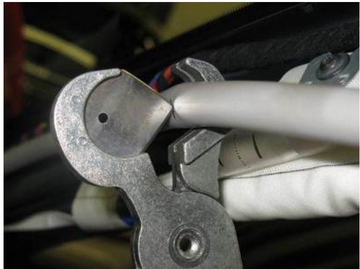
Figure 9. Cut the hose.
