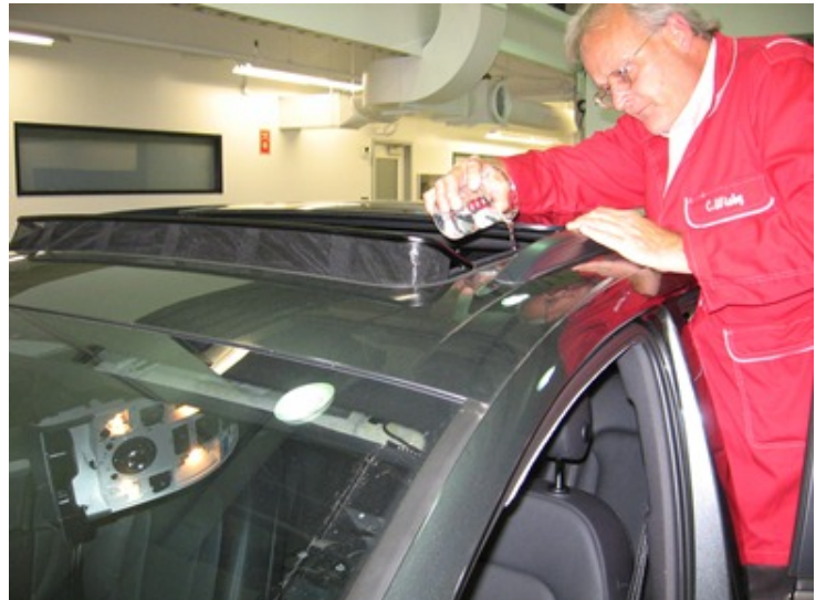
Figure 16. Test by pouring 200ml of water into the drain channels.
