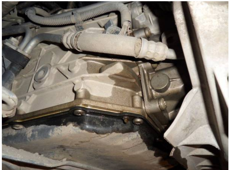
Figure 3. Leak between gearbox housing and intermediate housing.
