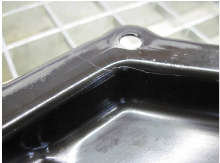
Figure 2. Crack in the oil pan.
