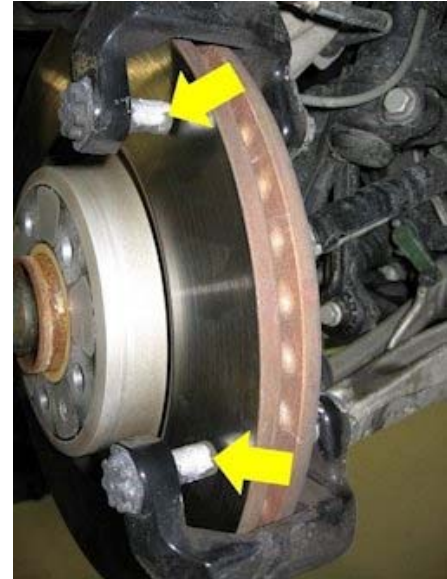
Figure 5. Caliper carrier guide pins with anti-seize ( G 052560A2 ) lubricant applied where the pads make contact.
