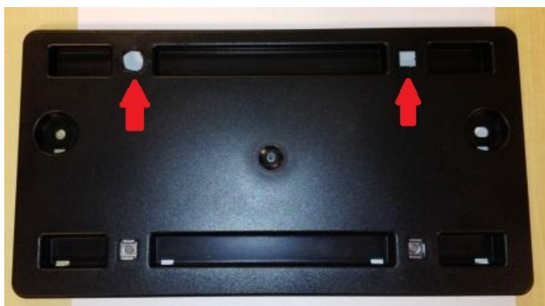
Figure 1. Damaged screw inserts
