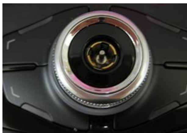
Figure 1. Control knob with missing joystick.
