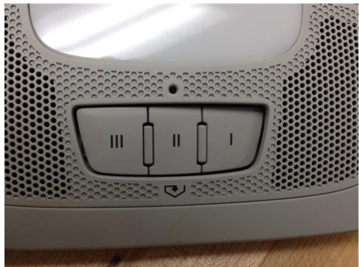
Figure 1. Homelink buttons pressed into the interior light assembly.
