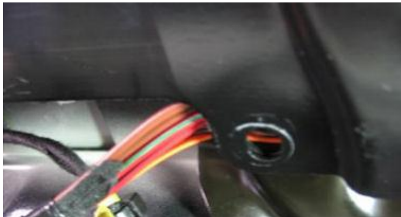
Figure 2. Closer view of wires that fell out of the sunroof frame groove and would become pinched between the sunroof frame and mounting bracket. Mounting bolt removed for demonstration purposes.
