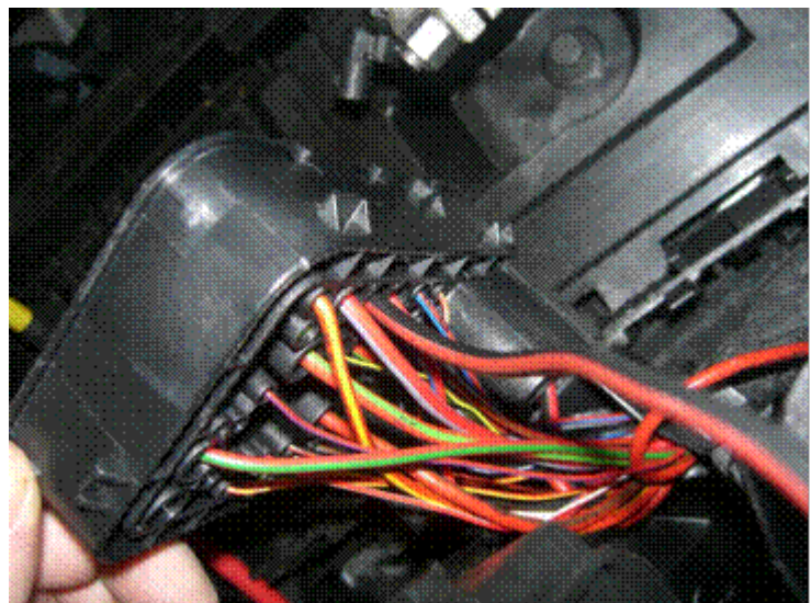
Figure 2. Overlay cable (red/black) inserted into T40 pin 27.
