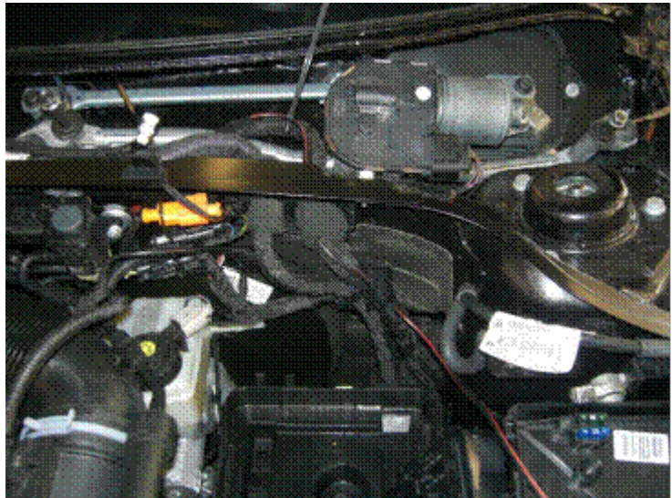
Figure 4. Routing up through plenum chamber.
