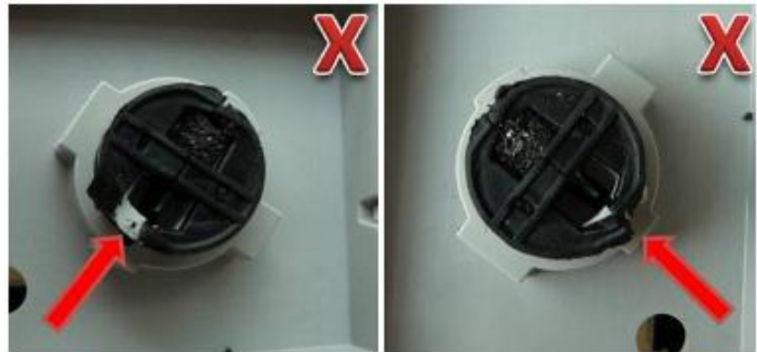
Figure 6. Examples of damaged seals
