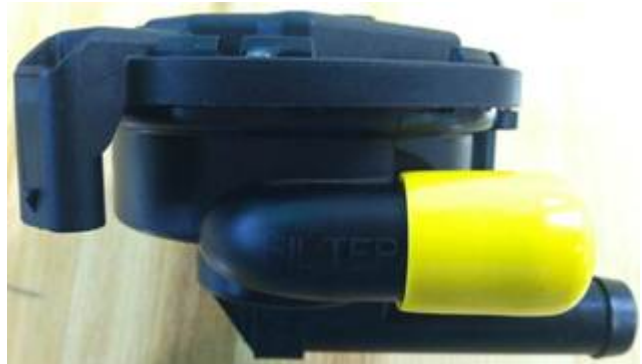
Figure 5. Example of plug inserted over the pressure sensor filter pipe
