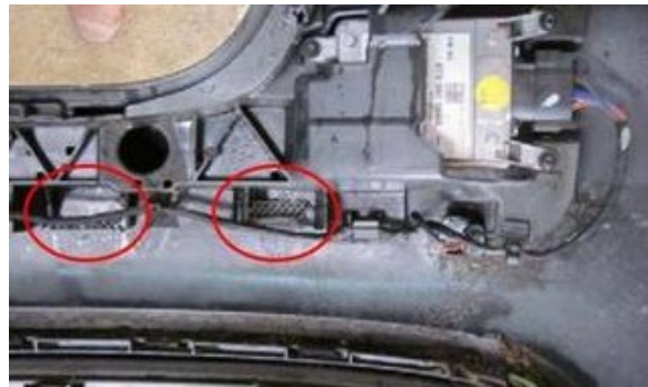
Figure 5. Bumper bracket weld locations with broken welds.
