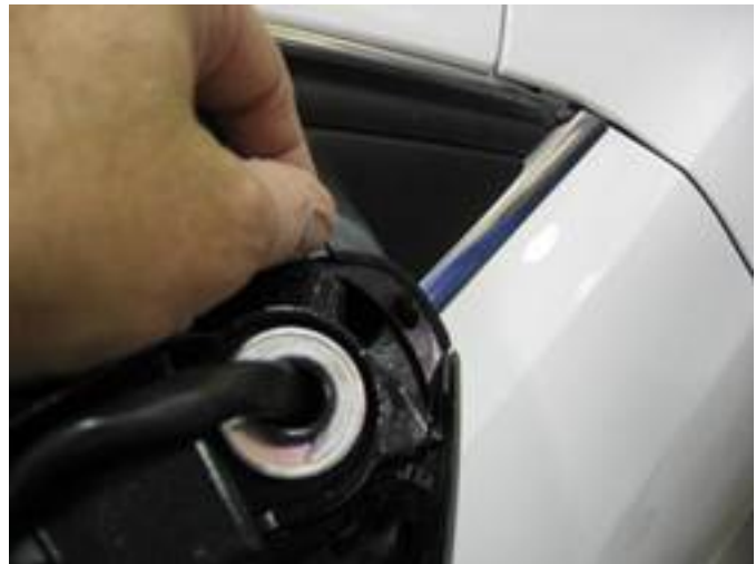
Figure 6. Application of felt tape.
