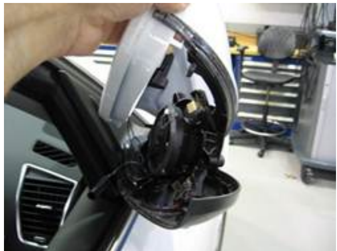
Figure 4. Removing the mirror cover.
