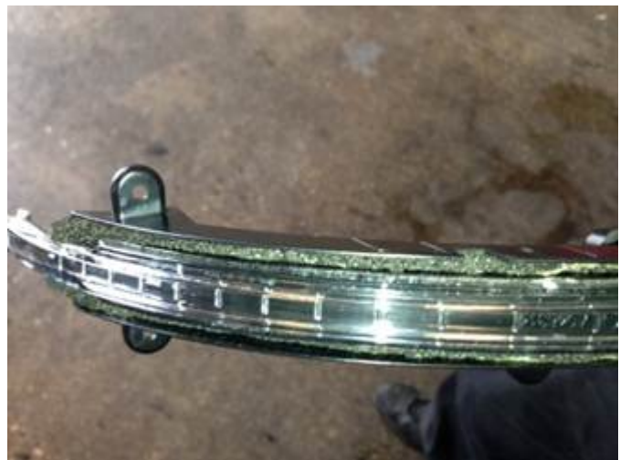
Figure 9. Turn signal lamp with sealing foam tape installed.
