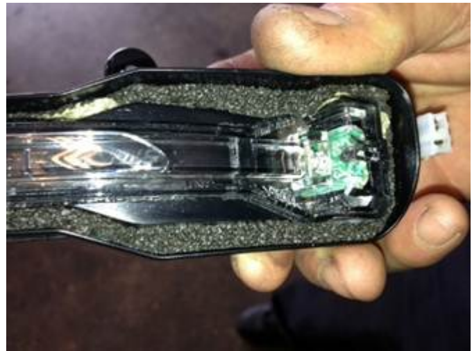
Figure 10. Turn signal lamp with sealing foam tape installed.
