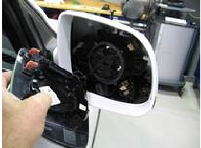
Figure 1. Exterior rear view mirror glass removed.
