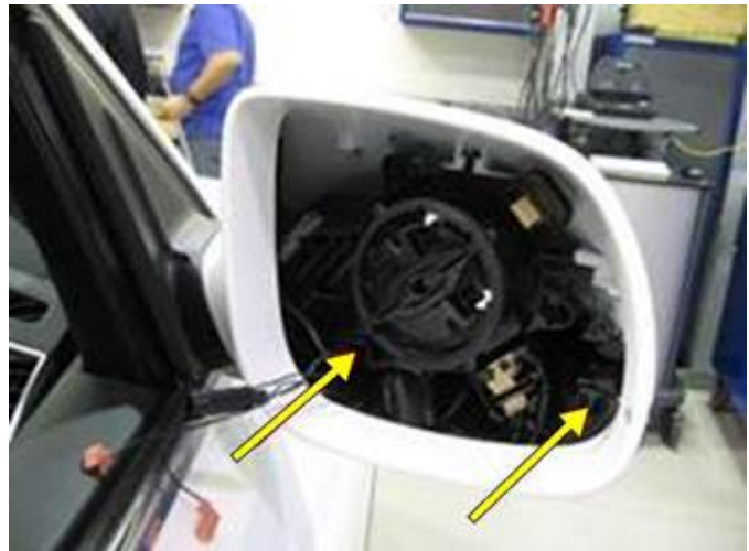
Figure 3. Location of the retaining clips.
