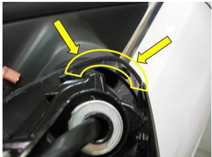
Figure 7. Felt tape applied.
