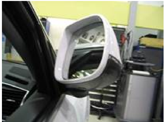
Figure 2. Exterior rear view mirror manually folded.
