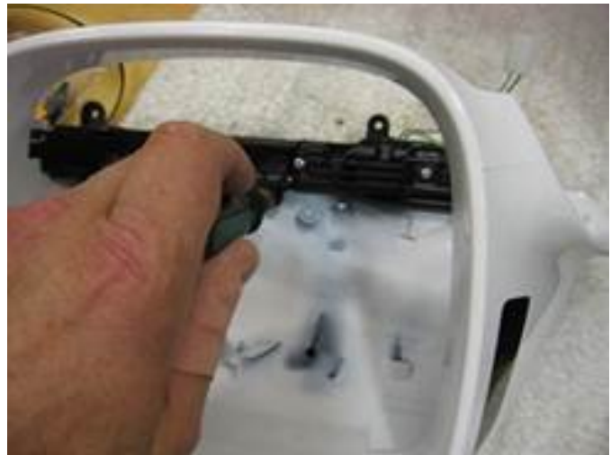
Figure 8. Removing the turn signal lamp.
