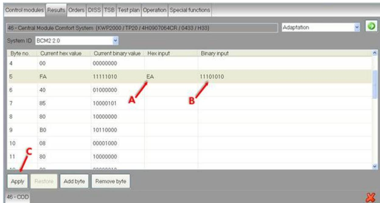
**Figure 5.** The new hex value input, EA (Arrow A), is shown in the **Hex input** column, and the new bit value input, 11101010 (Arrow B), is shown in the **Binary input** column. Click **Apply** (Arrow C) to update.
