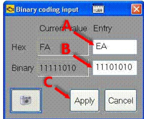
**Figure 4.** The Binary coding input pop-up window. In this example, Bit 4 in the Binary value (Arrow B) is changed from 1 to 0, so FA becomes EA (Arrow A). Click **Apply** (Arrow C) after making changes.
