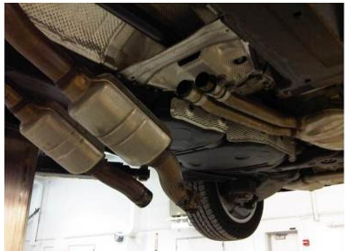
*Figure 4. Lowered catalytic converter pipes*
