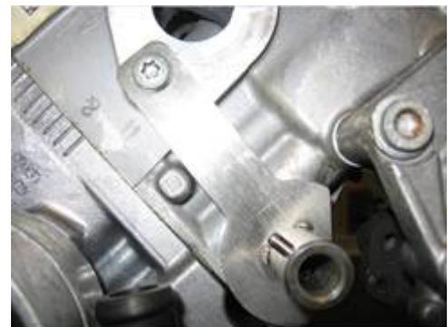
**Figure 11.** Engine adaptor on bank two.
