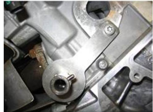
**Figure 10.** Engine adaptor on bank one.
