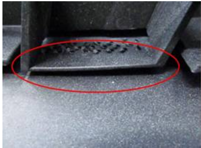
Figure 4. Loose mounting bracket.
