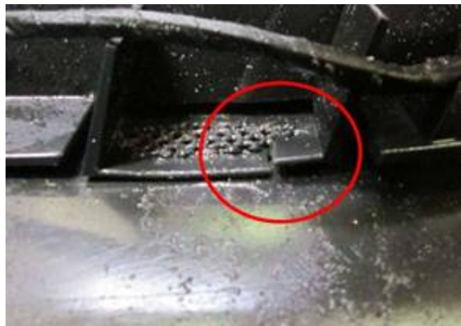
Figure 3. Broken mounting bracket
