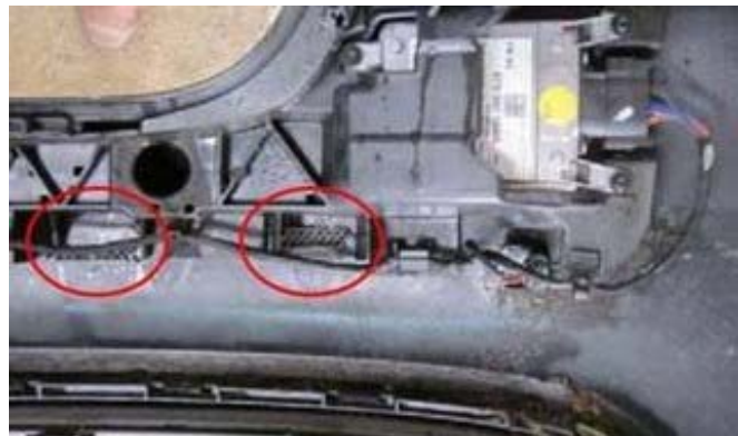
Figure 2. Mounting bracket for one of the ECUs.
