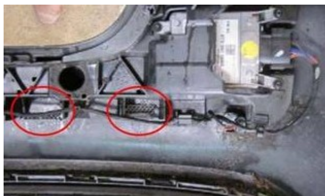
Figure 5. Bumper bracket weld locations with broken welds.
