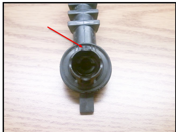
Figure 1. Incorrectly assembled drain hose, with locating tab pointing up.
