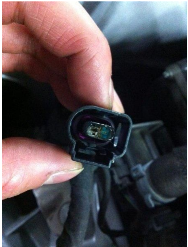
Figure 2. Corrosion formation on the connector pins.
