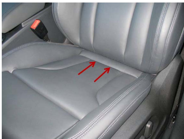
Figure 1. Arrows show area where additional fastening clips were added.
