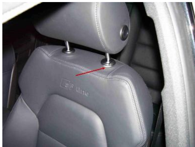
Figure 1. The head restraint feed-through hole, exposed.
